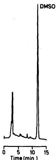
Fig. 1. Chromatogram of DMSO using ion-exclusion chromatography. Conditions: column, Bio-Rad Aminex HPX-87H (300 × 4.6 mm I.D.); eluent, 0.005 M orthophosphoric acid; flow-rate, 1.2 ml/min; detection, UV absorption at 195 nm; detector sensitivity, 0.05 a.u.f.s.; sample, 200 \mu l of a 5-ppm DMSO solution.
